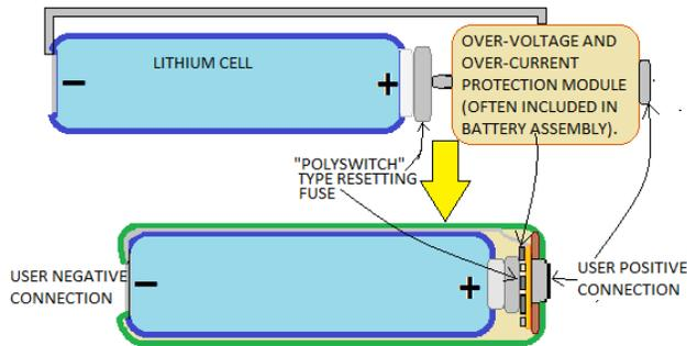
system fails. Far too many manufacturers depend on what is only intended as a safety backup to actually regulate the charging, using just a simple plugpack power supply.
