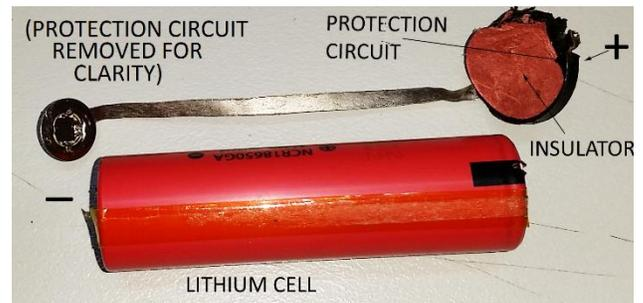
allows the circuit to monitor the battery voltage. This allows the cells to be removed and replaced like ordinary non-rechargeable cells. (The above example has had the outer wrapping removed to show the interior circuitry; normally it looks very similar to a standard 18650 cell).
