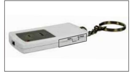
**Alarm Mode:** When the sensor detects movement whilst the unit is in alarm mode, it will not activate immediately. There is a thirty seconds delay, to allow you to use the remote control to disarm the sensor before it goes off. If the alarm unit is not disarmed within this thirty seconds delay, then the alarm will sound at full volume. The alarm can still be disarmed whilst the alarm is sounding by pressing the disarm button on the remote control.
