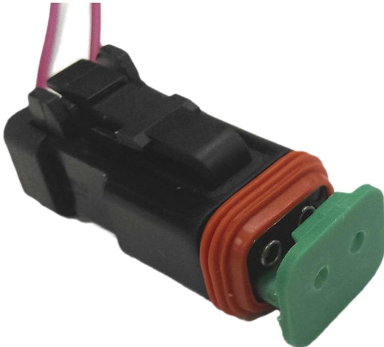
Once both of the female pins are in, you can fit the orange rubber grommet around the front of the plug, and slide the large green wedge with the face plate onto the front of the connector. This will tighten the pins against the case and clip everything together snugly. Once you get this on, you will not be able to remove it without destroying or scaring the plug.
